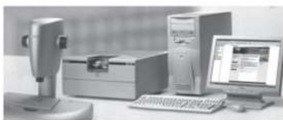
Fig. 13. Cerec inLab system – from left to right inEos extraoral Cerec in Lab with inbuilt dot scanner, PC computer with 3D software
